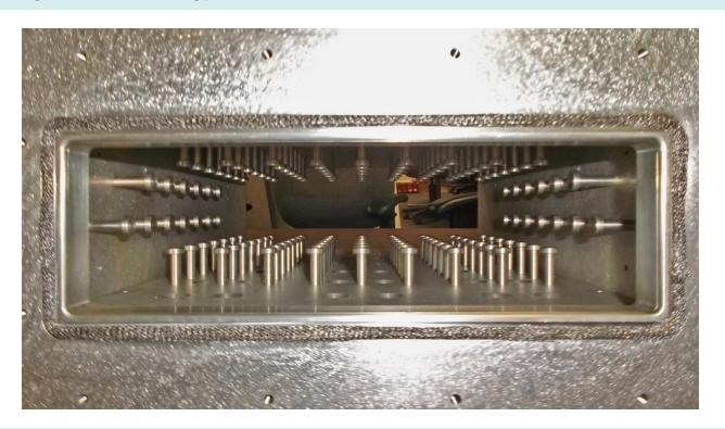
The small pegs inside the waveguide entrance to the cell act like a choke at microwave frequencies. They are called image-plane monopoles, and are spaced a quarter-wave apart. They are just
